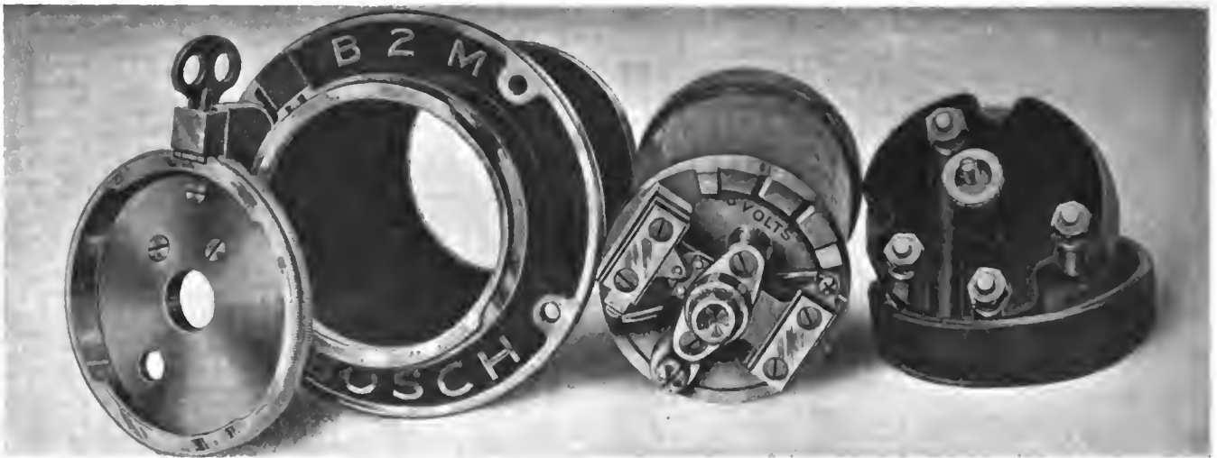
Fig. 1—Parts of the synchronous coil of Bosch Dual Ignition System disassembled to show construction.
